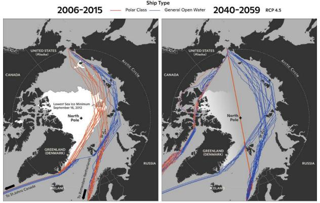
**Fig. 1.** Model of maritime ship-traffic in the Arctic Ocean (Smith and Stephenson 2013), predicting trade routes that will open as sea ice diminishes through mid-21st century with polar-class ships that are ice-strengthened (orange) according to the International Association of Classification Societies (IACS) and other ship types that are designed for open water (blue).
